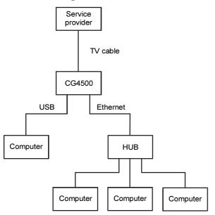
Multiple users are supported with a single user attached to the USB port and the remaining (up to 31) users connected to the Ethernet hub.
