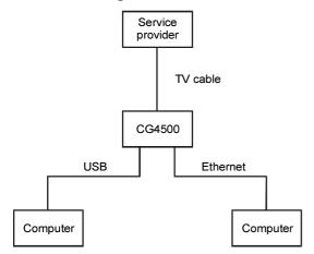
Multiple user configurations can include Ethernet and USB connections.
