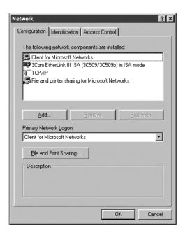
The CG4500 contains all necessary software. You don't need to configure the CG4500, but you must configure your computer for TCP/IP and check for an IP address. Your service provider may provide additional instructions for setting up your computer. The following basic instructions are for Windows 95 or Windows 98. Use Microsoft online help to install and configure hardware for Windows 2000 and Windows Me. If you are using a different operating system, refer to that user guide.
