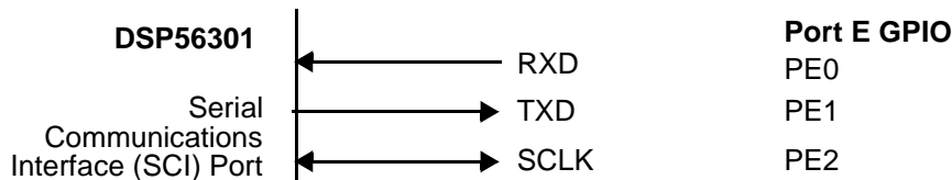
Figure 5-5. Port E Signals
