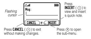
When you enter text using the standard tap method (see page 21), the flashing cursor changes to a *block cursor*, and the soft key functions change:
