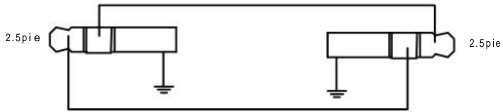
Figure 2-16 Cloning Cable Schematic
