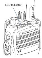
**Blinking yellow** – Radio is scanning for activity or receiving a Call Alert.
