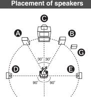
The front, center, and surround speakers should be placed at approximately the same distance from the seating area. The angles in the diagram are approximate.
