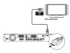
• The arrow on the cable connector body should be face down for correct alignment with the connector on the recorder.
