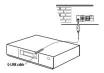
See the manual that came with your cable box if you're not sure where the IR receiver is on the front panel. Alternatively, experiment with the remote control, operating it from very close range until you find the place where the receiver responds.
