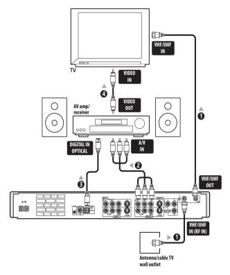
1 Connect RF antenna cables as shown.
