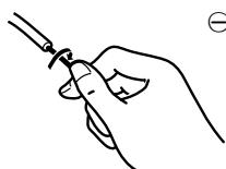
2. Push the lever, insert the cable into the hole, and release the lever.
