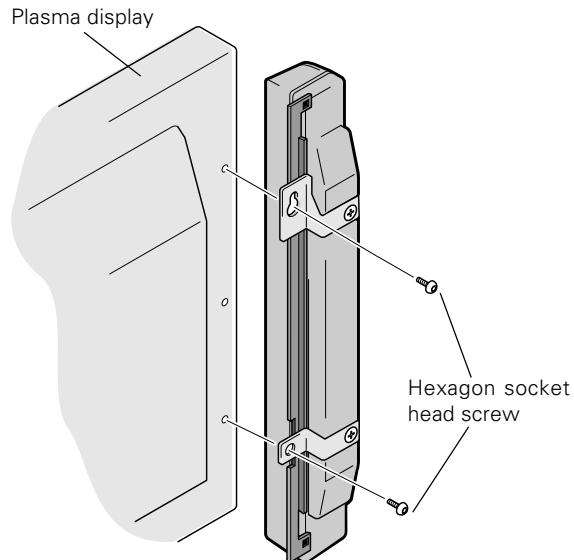
① To attach the speakers to the display, start by placing the upper screw where indicated, tightening until there is a small space of about 5mm between the head of the screw and the display.
