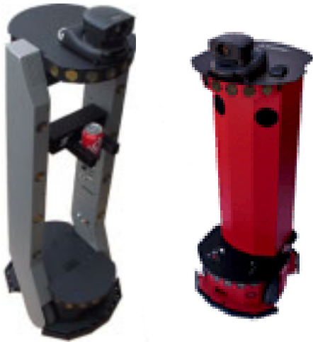
Figure 7. Nearly identical to its research predecessor (right), the Performance PeopleBot (left) sports an attractive body design and bundled systems, including integrated Gripper, for commercial-consumer human-interaction applications.
