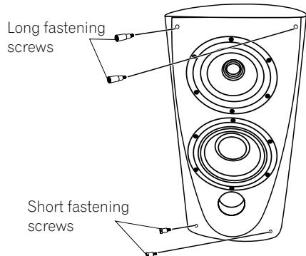
**2 Line up the holes on the grille with the protruding ends of the screws on the front of the speaker and press firmly.**
