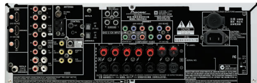
Rear Panel of VSX-918V (Same for VSX-818V, except it does not have SR+ terminals)
