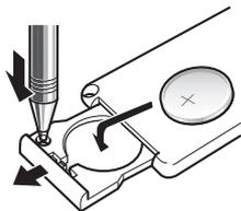
**Remove the cover on the back of the remote controller unit and insert the battery with the (+) and (-) poles pointing in the proper direction.**
