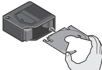
Align the disc tray with the left and right grooves, and push it in until you hear it click.
