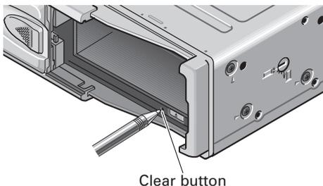
After connecting everything up, press the clear button with the tip of a pencil. If the power will not switch on, or if the CD player does not operate, when the button on the control unit is pressed, or if the control unit display is incorrect, press this button with the tip of a pencil to restore normal operation. (This button is located inside the door.)
