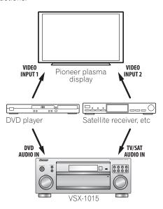
To make the most of the SR+ features, you should connect your source components (DVD player, etc.) in a slightly different way to that described in this chapter. For each component, connect the video output directly to the plasma display, and just connect the audio (analog and/or digital) to this receiver.
