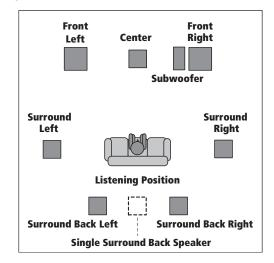
The diagrams below show suggested surround and surround back speaker orientation. The first diagram (*fig. A*) shows orientation with one surround back speaker (or none) connected. The second (*fig. B*) shows orientation with two surround back speakers connected.
