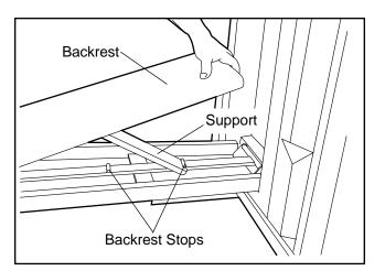
of the backrest stops as shown. **Make sure that the** support is resting against one of the backrest stops.
