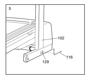
Remove the backing from the Adhesive Clip (129).
