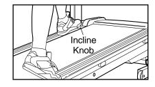
Using your left foot, press down the incline knob until the desired incline is reached. To decrease the incline, **stand with your right foot near the front of the right foot rail** while pressing down the incline knob. Note: It may be helpful to step off the treadmill when pressing down on the incline knob to decrease the incline.
