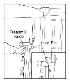
Slowly release the knob. Make sure that the lock pin is inserted into the hole in the treadmill frame.
