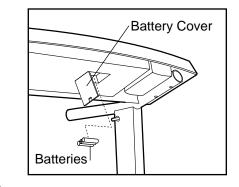
the negative ends of the batteries (marked "–") are touching the springs in the battery compartment. Close the battery cover.
