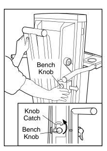
**position.** Note: It may be necessary to push on the leg while you slide the knob to the "bench" position .
