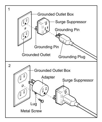
The green-colored rigid ear, lug, or the like extending from the adapter must be connected to a permanent ground such as a properly grounded outlet box cover. Whenever the adapter is used it must be held in place by a metal screw. **Some 2-pole receptacle outlet box covers are not grounded. Contact a qualified electrician to determine if the outlet box cover is grounded before using an adapter.**
