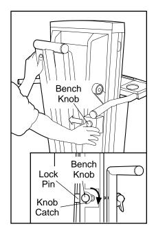
in the hole into the bench frame. Pivot the knob catch down around the knob.
