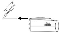
To adjust the mounting angle, remove the detector from the bracket. Then, remove the bracket from the windshield and adjust it by carefully bending it.
