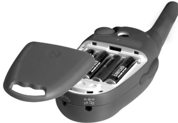
5. Replace the cover and push the latch up until it clicks. Then rotate **Off** ◀ counterclockwise until it clicks to turn on the radio.
