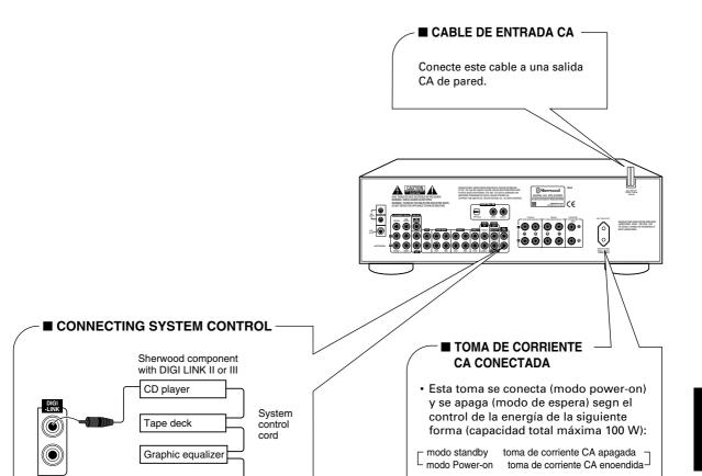
Connect this jack to the DIGI LINK jack of the external Sherwood component that uses the DIGI LINK II or III remote control system.
