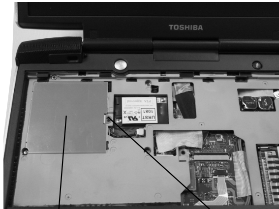
Mini PCI cover M2.5x4 security torx screw
