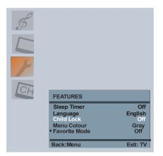
When **Child Lock** is selected, a reminder will appear when any of the topl buttons are pressed. Once the television has been switched off it can ONLY be brought out of standby using the remote control.
