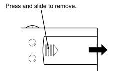
2 Install two "AA" size batteries. Match the + and – signs on the batteries to the signs on the battery compartment.
