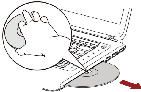
Figure 4-7 Removing a CD/DVD
