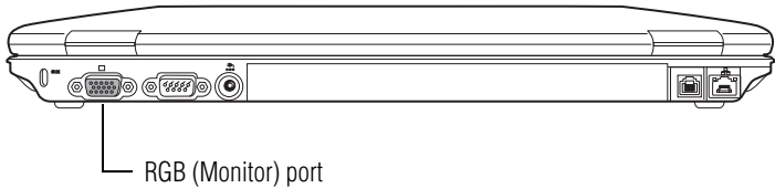
(Sample Illustration) Video port on back of system
