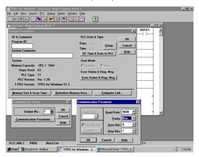
Click on the "Computer Link" button in the System Parameters screen, and the "ComputerLink Setup" menu will appear. Select a station number for the PLC, then click the "Communication Parameter" button. Select "NON" parity setting, and then click the "OK" buttons. When the "Write OK" screen appears, click "OK."
