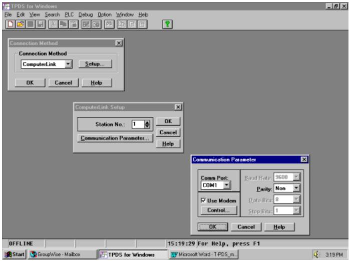
Go to the Options/Communication menu and set the above parameters. Remember that we set the PLC Computer Link station address as 1 on the previous page. Be sure to select "**NON**" parity here. Check the "**Use Modem**" box and click the "**Control**" button to get to the next screen.
