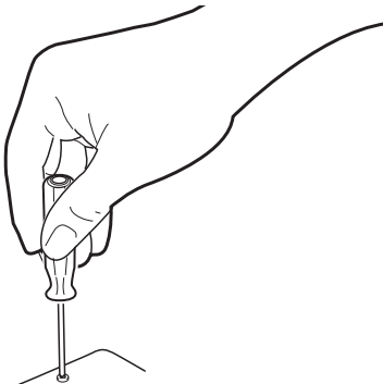
(Sample Illustration) Removing the memory module slot cover
