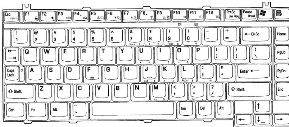
Figure E-2 Keyboard layout (for US)
