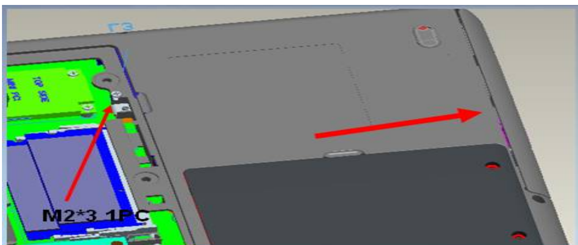
Figure 4-18-2 Remove the screw on ODD Bezel and ODD
