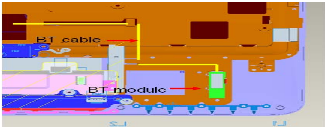
Figure 4-19-1 Remove the Bluetooth cable
