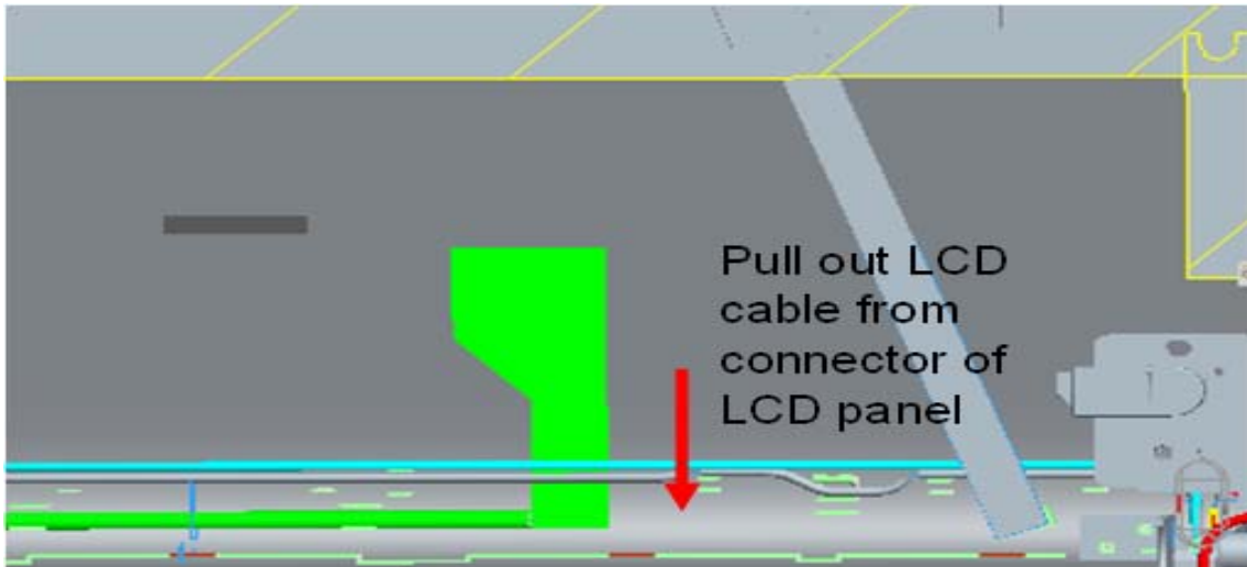
Figure 4-8-6 Remove the LCD cable from LCD panel
