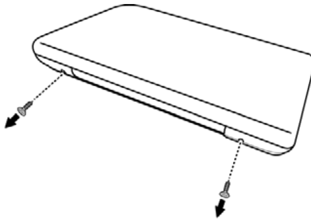
Figure 4-32 Removing the rear screws
