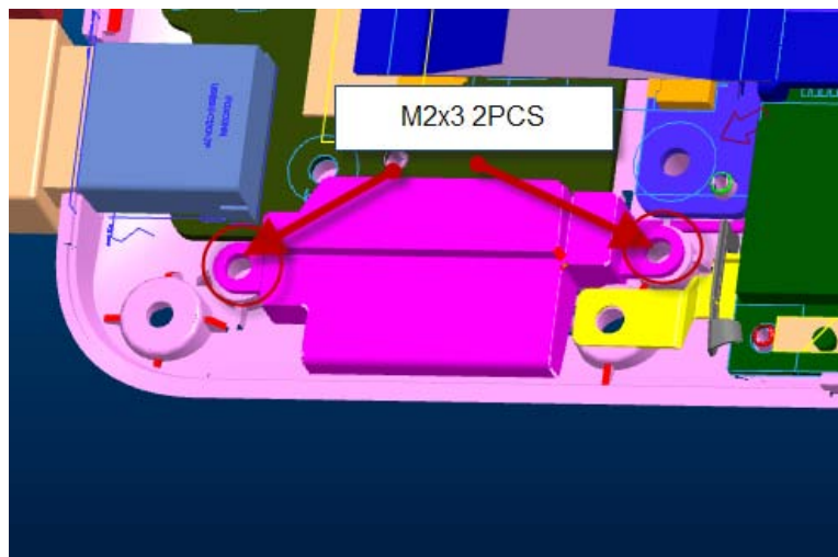
Figure 4-17-1 Remove the securing screws at left side.
