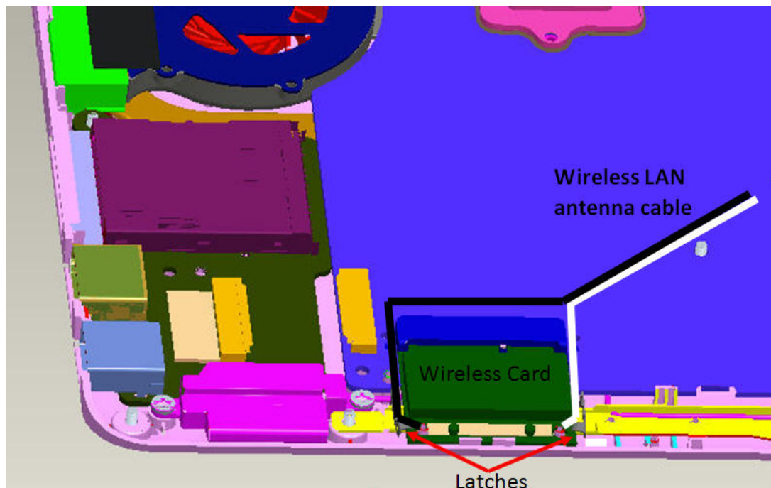
Figure 4-6-1 Remove a wireless LAN card
