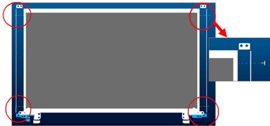
Figure 4-14-5 Remove the LCD hinge
