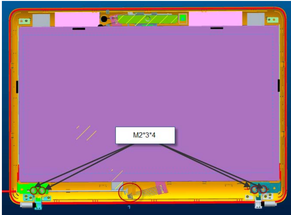
Figure 4-14-2 Remove screws securing the LCD
