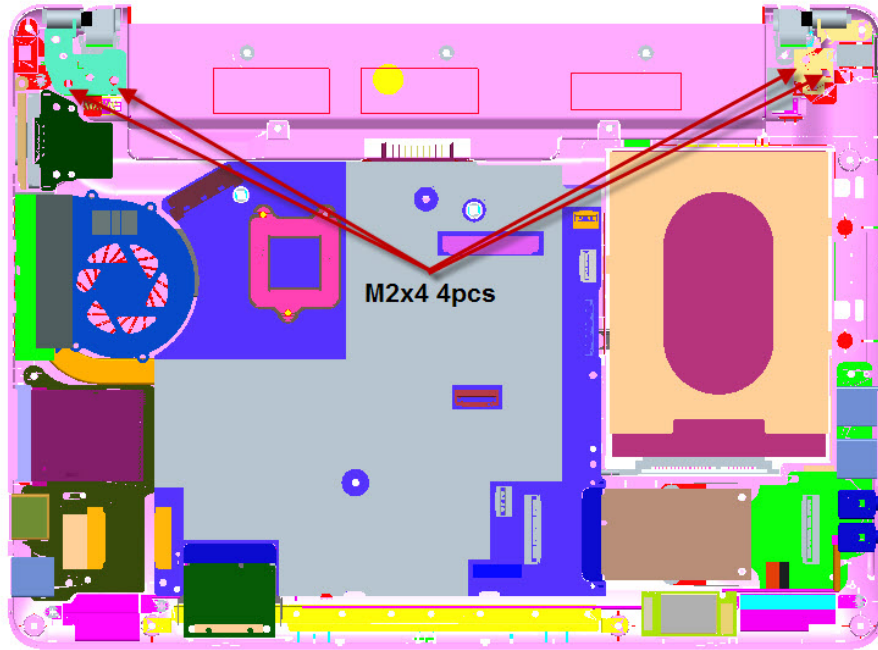
Figure 4-8-8 Remove the hinge screws
