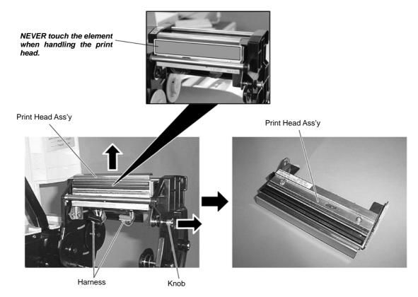
4) Replace the Print Head with a new one, and then reassemble in the reverse order of removal.
