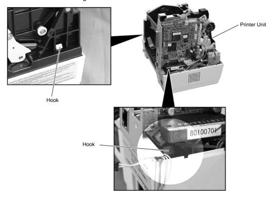
7) Detach the Printer Unit from the Bottom Cover.
