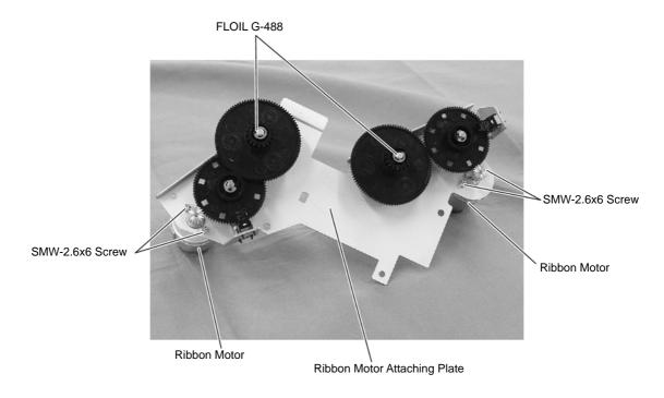
4) Replace the Ribbon Motors with new ones, and then reassemble in the reverse order of removal.
