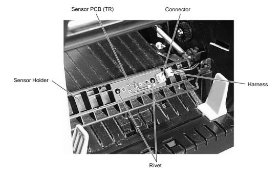
6) Replace the Sensor PCB (TR) with a new one, and then reassemble in the reverse order of removal.
