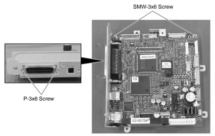
11) Remove the SMW-3x6 screw, N-3 Nut and Ground Plate.
