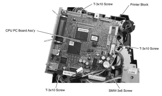
10) Remove the four screws (SMW-3x6 and P-3x6) and detach the CPU PC Board from the PC Board Attached Plate.
