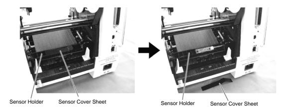
4) Release the Sensor Holder while spreading the tabs of the Sensor Holder. Be careful not to break the tabs when spreading them.
