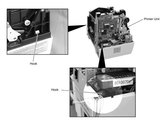
5) Detach the Printer Unit from the Bottom Cover.
