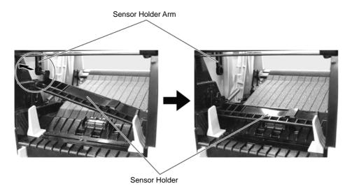
3) Remove the Sensor Cover Sheet from the Sensor Holder.
