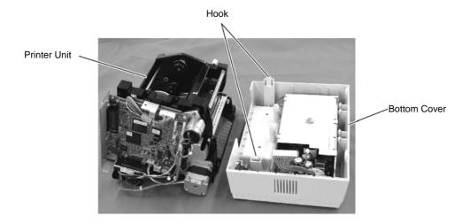
8) Disconnect the harness from the Sensor PCB (LED) which is attached to the bottom of the Printer Unit. Then remove the Rivet to detach the Sensor PCB (LED) from the Printer Unit.
