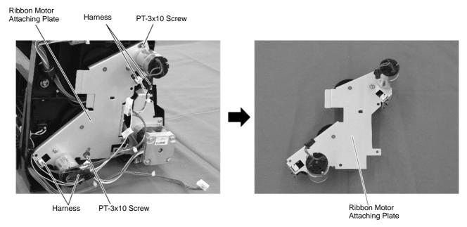
Remove the four SMW-2.6x6 screws to detach the two Ribbon Motors from the Ribbon Motor Attaching Plate.
