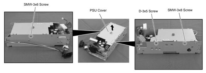
9) Disconnect the Power Harness from CN4 on the PS Unit. Remove the SMW-4x8 screw to release the Ground Wire of the Inlet Ass'y.
