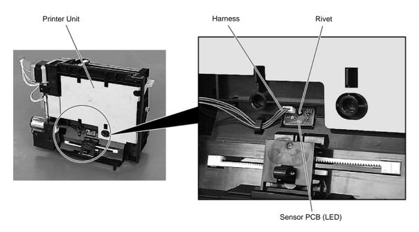
9) Replace the Sensor PCB (LED) with a new one, and then reassemble in the reverse order of removal.
