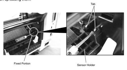
5) Disconnect the harness from the Sensor PCB (TR), and remove the Sensor PCB (TR) from the Sensor Holder by releasing the two Rivets.
