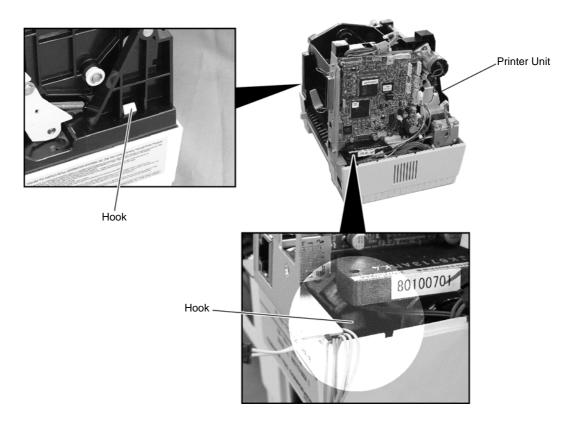
8) Detach the Printer Unit from the Bottom Cover.
