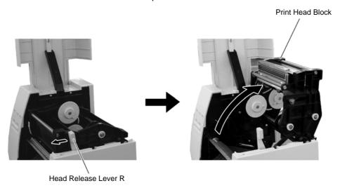
Disconnect the two Print Head Harnesses. Then, pull the Print Head Ass'y upward while pulling the Knob.
