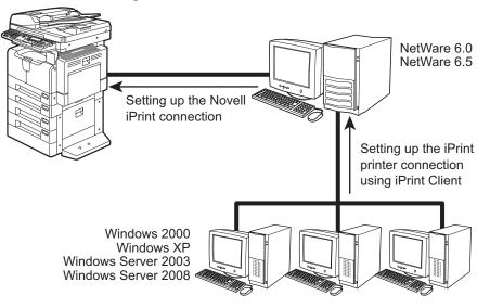
Connecting with a Novell iPrint Environment over TCP/IP Network
