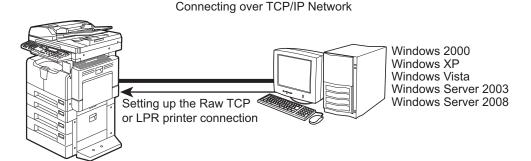
This equipment can be used with Raw TCP or LPR printing connection for Windows 2000, Windows XP, Windows Vista, Windows Server 2003 and Windows Server 2008. The Raw TCP printing connection is recommended for Windows 2000, Windows XP, Windows Vista, Windows Server 2003 and Windows Server 2008.
