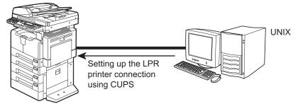
This equipment can be used with the LPR printer connection when the UNIX workstations computers and the equipment are connected over the TCP/IP network.
