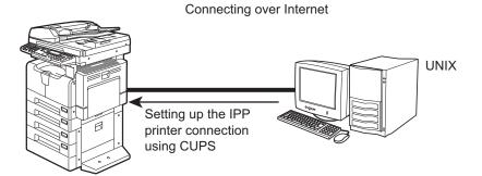
This equipment can be used with the IPP printer connection for UNIX workstation in a TCP/IP network using CUPS. Even though IPP printing can be used in a local area network, this method is commonly used to print over the Internet. If you allow IPP printing through the Internet, you must configure the DNS server to enable users to access this equipment over the Internet using the HTTP protocol. This is useful when users want to print to this equipment from outside the local area network.
