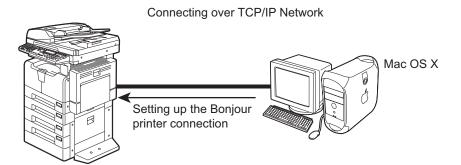
This equipment can be used with the Bonjour printer connection when the Macintosh computers of OS X and the equipment are connected over a TCP/IP network.
