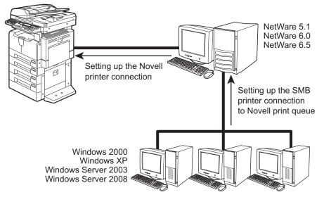
When you want to manage the print jobs in the NetWare print server instead of directly printing to this equipment, an administrator must configure the NetWare print servers and this equipment.
