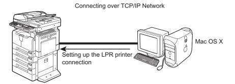
This equipment can be used with the LPR printer connection when the Macintosh computers and the equipment are connected over the TCP/IP network.
