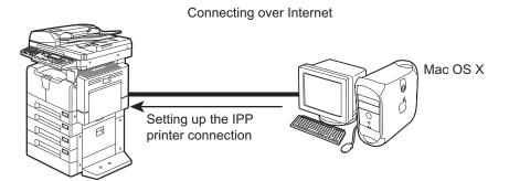
This equipment can be used with the IPP printer connection for Mac OS X in a TCP/IP network. Even though IPP printing can be used in a local area network, this method is commonly used to print over the Internet. If you allow IPP printing through the Internet, you must configure the DNS server to enable users to access this equipment over the Internet using the HTTP protocol. This is useful when users want to print to this equipment from outside the local area network.
