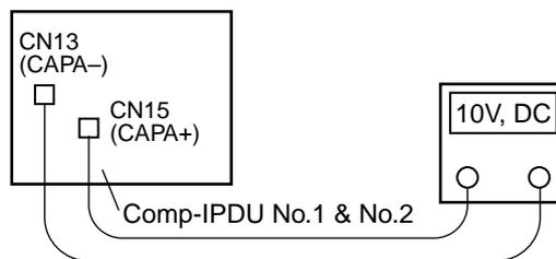
COMP-IPDU No. 1 and COMP-IPDU No.2 have the same electric potential, measure both.
