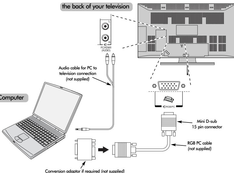
Connect the PC cable from the computer to the PC terminal on the back of the television.
