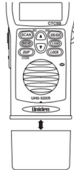
2. Use a coin to turn the screw that connects the battery pack to the **UH-052XR**. Be sure the battery pack fits tightly against the **UH-052XR** body.
