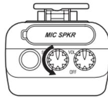
To set the "Squelch Gate" to the desired level, turn **[SQ]** counter-clockwise until you hear noise. Then turn the **[SQ]** clockwise just until the noise stopped. Now only the desired signal can get through.
