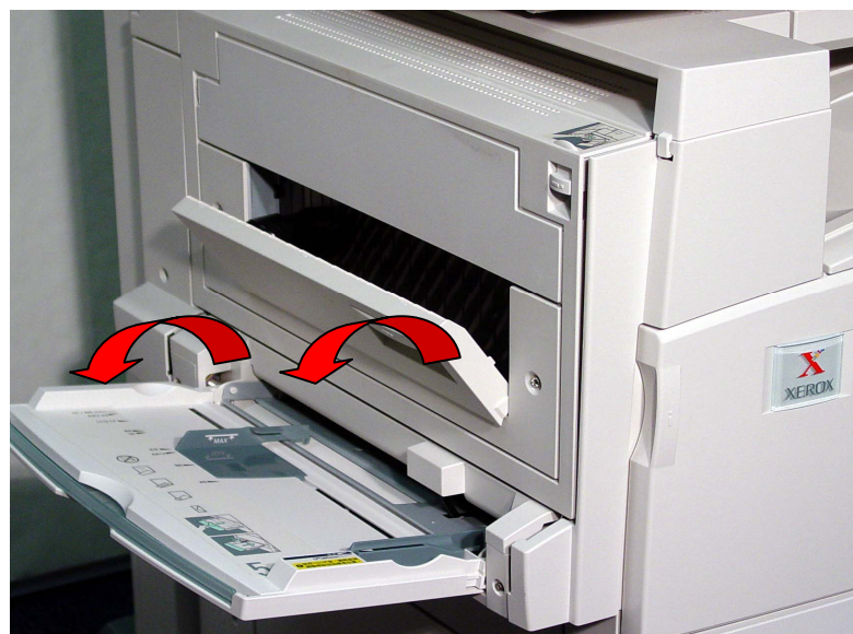
Fig. 4 Duplex Module Cover Open the tray 5 (Bypass) and gently open the duplex module cover.
