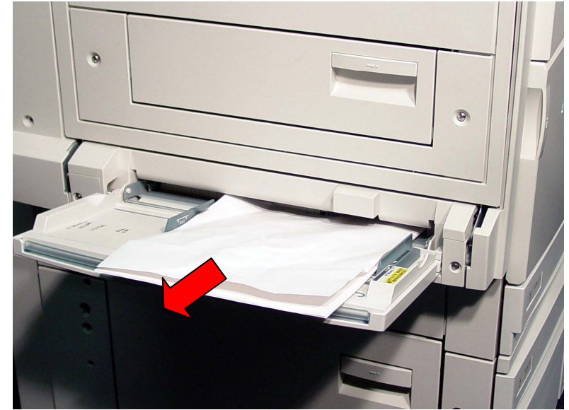
Fig. 6 Tray 5 (Bypass) Inspect the inside (paper feed entrance) of Tray 5 (Bypass), and remove any jammed paper.
