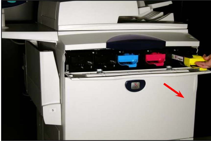
Fig. 3 Pull the toner cartridge indicated in the message on the display out.
