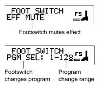
Use the REV TIME control to switch between the EFF MUTE and PGM SEL functions. If you select the former, the REV500's effect output will be suppressed when you depress the footswitch. Depress the footswitch again to release the effect mute.
