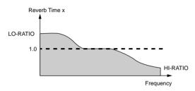
The four PARAMETER EDIT controls on the REV500's front panel let you adjust the basic program parameters quickly and easily. When you rotate one of these controls, the program information in the LCD (shown above) will be replaced by a graphic display indicating how the changes you've made have affected the parameter in question. (The display will return to normal a few moments after you stop turning the control.)
