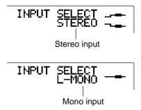
Use the REV TIME control to switch between the STEREO and L-MONO input settings. When you have made your setting, press one of the PROGRAM keys to exit the utility mode.
