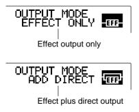
Use the REV TIME control to switch between the EFFECT ONLY and ADD DIRECT output mode settings. When you have made your setting, press one of the PROGRAM keys to exit the utility mode.
