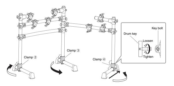
4. Loosen the clamp (5), (6) and (7) bolts, adjust the position of the cymbal arms and the drum trigger module arm, and then tighten the bolts again so they are secure.
