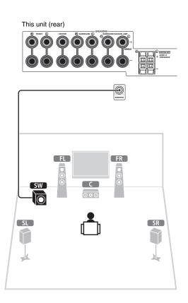
Use an audio pin cable to connect the subwoofer (SW).
