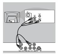
Use the composite video cables (yellow) to connect the DVD player's VIDEO(CVBS) jack to the video input jack(or the labled as A/V in,Video In or Composite) on the TV(cable supplied).
