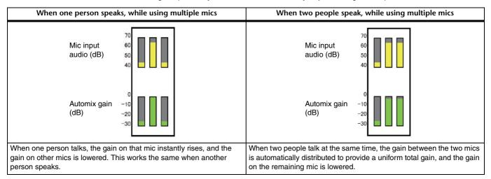
Unlike limiters or auto-level controllers, the Dugan speech system lets the engineer control individual levels as usual, even when more than one person is talking at the same time. Also, the audio on the mics is detected and the gain is automatically distributed when no one is talking, so the faders can be left up.
