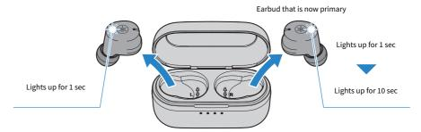
If successfully connected, you will hear the "Connected" audio message in the earbud. Pairing is now complete.
