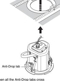
When all the Anti-Drop tabs cross over the O-ring, the speaker is held temporarily.
