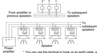
\* You can use this terminal to hook up an earth cable, as necessary
