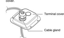
If it is difficult to pass all the cables through a single cable gland, open the hole in the terminal cover and attach a commercially available
