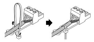
Trim any excess part of the cable tie as necessary.
