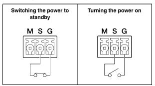
When the power is set to standby via the [REMOTE] connector, turning on the power switch will place the unit in standby mode.
