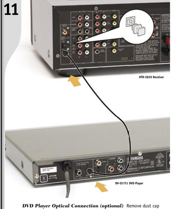
on optical input as shown on inset. Connect optical cable (not included) to receiver. Connect optical cable to DVD player from receiver.
