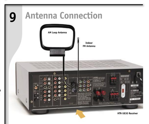
Connect Antennas to Receiver Locate AM loop antenna and indoor FM antenna. Keeping receiver unplugged, connect as shown. For more information about obtaining clear reception and grounding, see your Owner's Manual.
