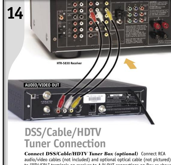
audio/video cables (not included) and optional optical cable (not pictured) to "DTV/CBL" terminals on receiver to A/V OUT connections on Box as shown.
