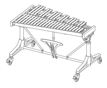
8. Lock the casters by pressing the stoppers of the left and right casters.
