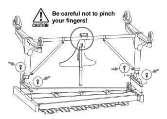
6. To prevent the pedal from moving uncontrollably, secure the damper by hooking the damper belt tip to the hook of the main unit.
