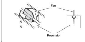
We recommend that you set the fan to a vertical position, to ensure the strongest resonator effect.
