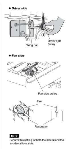
4-8. Tighten the wing nut firmly.
