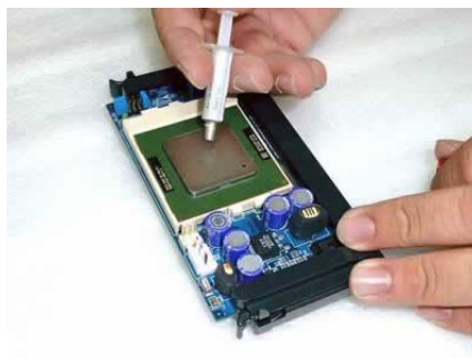
Applying thermal compound to the processor.
