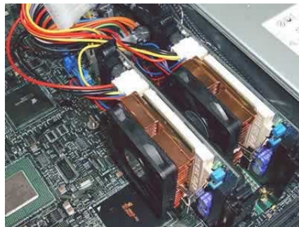
Dual PL-P3/SMPs, installed and connected.
