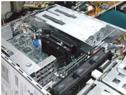
The original Slot 1 processors. Be sure to disconnect the system power before continuing with your processor upgrade.
