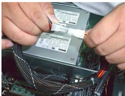
Connecting the PL-P3/SMP's power cable to the WTX power supply connector.
